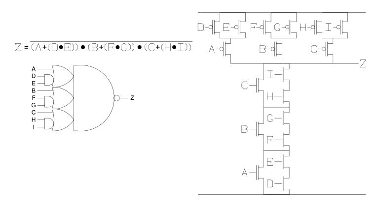
No possible path through p-transistors. No re-arrangement will create a solution!
