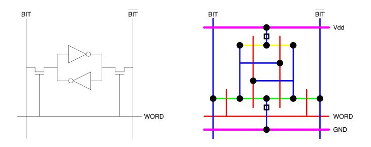
Standard 6 transistor static RAM cell.
