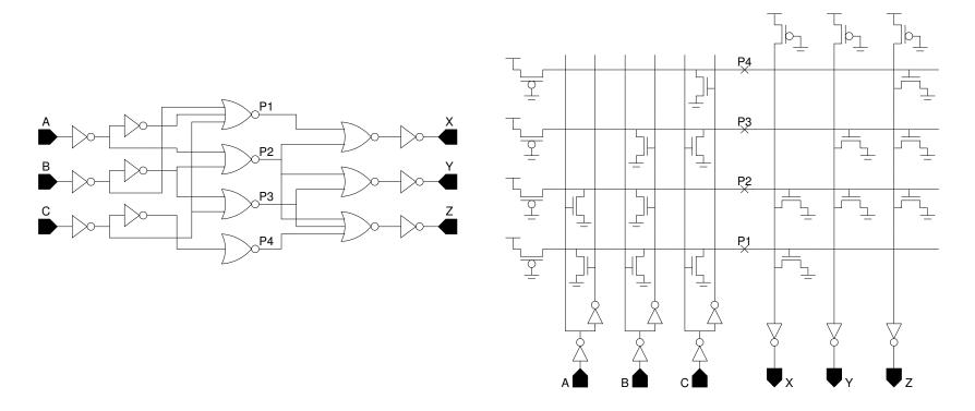
• A regular layout is employed, with columns for inputs and outputs and rows for intermediate expressions.
