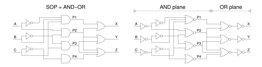
Most PLA structures employ pseudo-NMOS NOR gates using a P-channel device in place of the NMOS depletion load.
