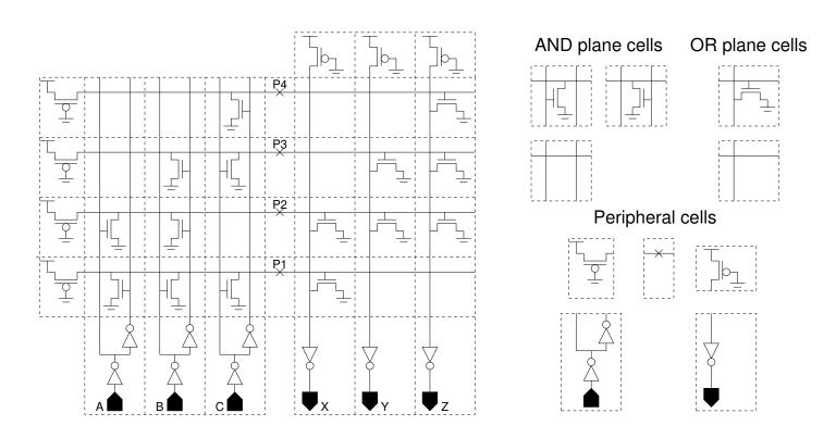
• Layout is simply a matter of selecting and placing rectangular cells from a limited set.
