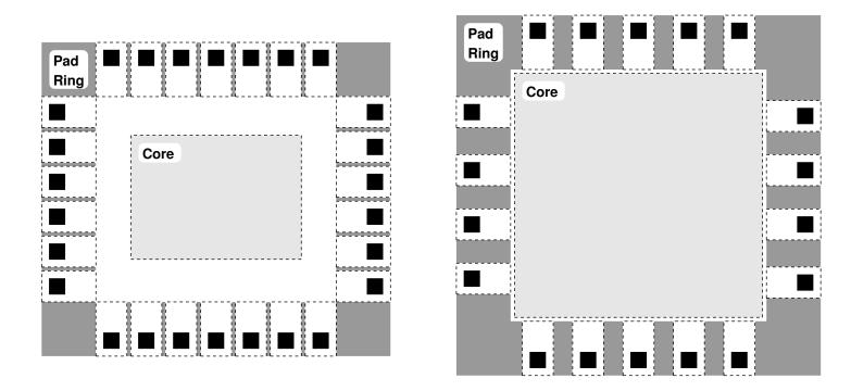
**Pad Limited:** small core and/or many pads minimum pad to pad distance – gaps around core
