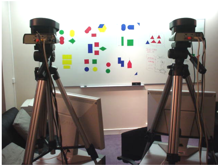
Figure 1: The 'Talking Heads' experiment featured pan-tilt cameras oriented towards a white board on which geometric figures were pasted. Agents used these cameras to play lexical language games drawing attention to a chosen topic.
